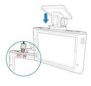
Connect the B+ power cable to the DC-IN input terminal of themain unit.
