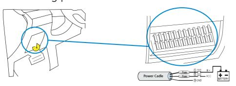
The fuse box is usually located under the dashboard of driver's seat.
